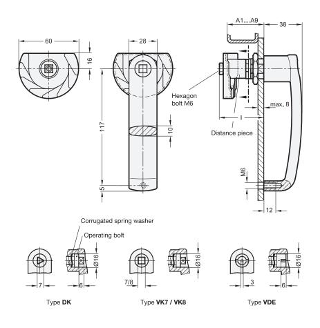
\* Complete with type index of the latch
